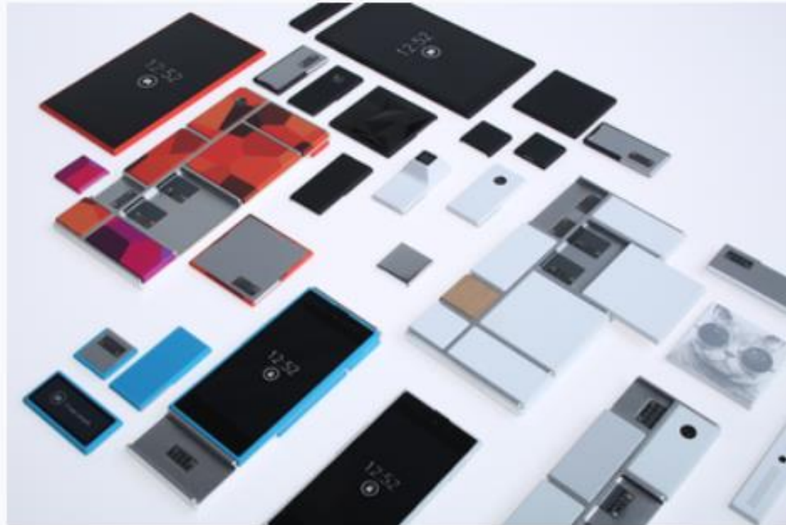
Ara smartphones with individual modules separated
